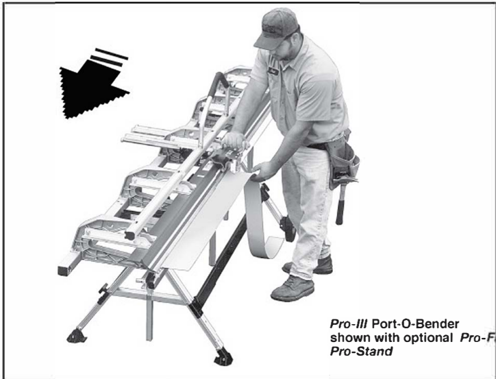
Figure 3. Use proper technique to push CUT-OFF through the material with a smooth, constant motion from right to left. Do not stop in the middle or cut with a back and forth motion. Use a piece or two of scrap material to practice.
