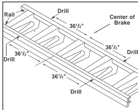
**2** Invert Brake. From center of Brake, measure outward along each rail 36 1/2" and drill one pilot hole in center of each rail using an 11/64" drill bit.
