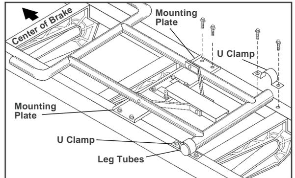
**3** Set legs onto Brake with leg tubes near drilled pilot holes. Place "U" clamps over leg tubes, align holes and install sheet metal screws. Drill remaining holes through clamps and install screws. Install screws also in mounting plates as shown.
