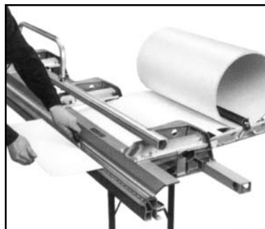
Fast, simple one-man operation. Roll out and cut squarely to your exact length.
