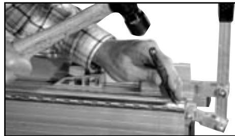
5 After replacement, "Center Punch" Stainless Bending Edge on ends to prevent possible sliding.
