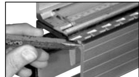
6 Punch Vinyl When Vinyl Protecto Strip is in place "center punch" both ends to prevent slip-page.
